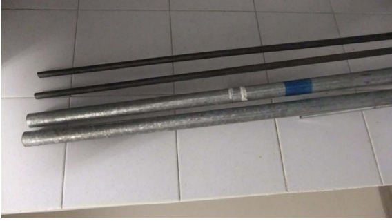
Fig. 11. Galvanized steel pipes, reinforcing rebars and iron rods used for experiments.
